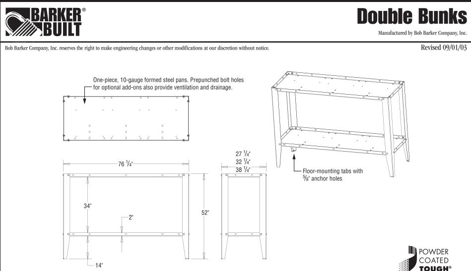
Double bunks should be securely anchored to the floor. Each bunk requires 4 anchors for floor attachment.
